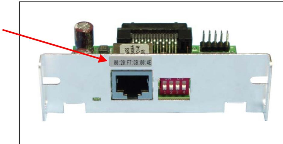
The Ethernet IV module will have the 01-02 assembly numbers, The Serial Number and firmware version number located on the back of the Panel.
