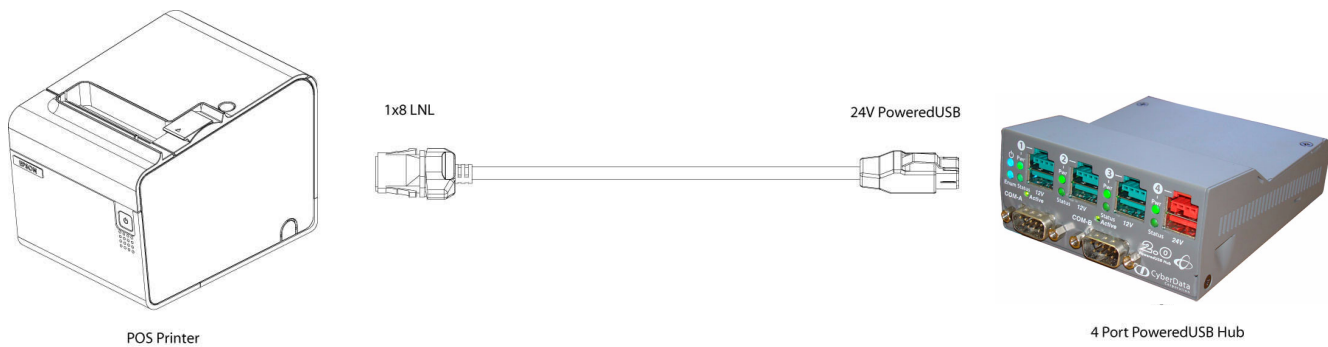
Figure 2-13. Cable, +24V PoweredUSB to 1x8 PoweredUSB
