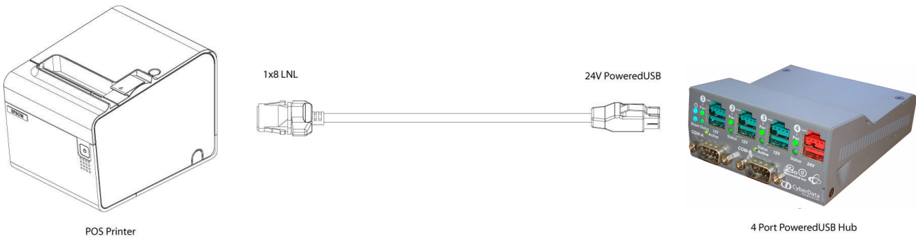
Figure 2-13. Cable, +24V PoweredUSB to 1x8 PoweredUSB
