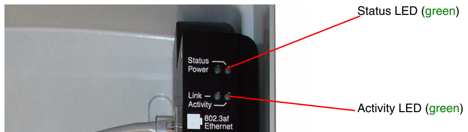
Figure 2-6. Loudspeaker Amplifier LEDs—Status and Activity
