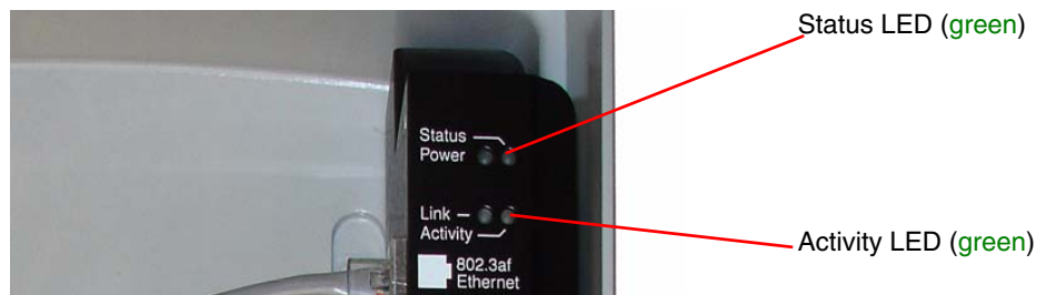
Figure 2-6. Loudspeaker Amplifier LEDs—Status and Activity
