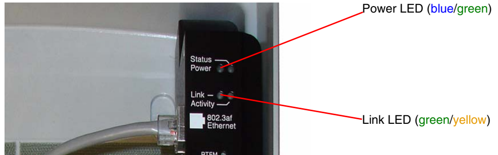
Figure 2-5. Loudspeaker Amplifier LEDs—Power and Link
