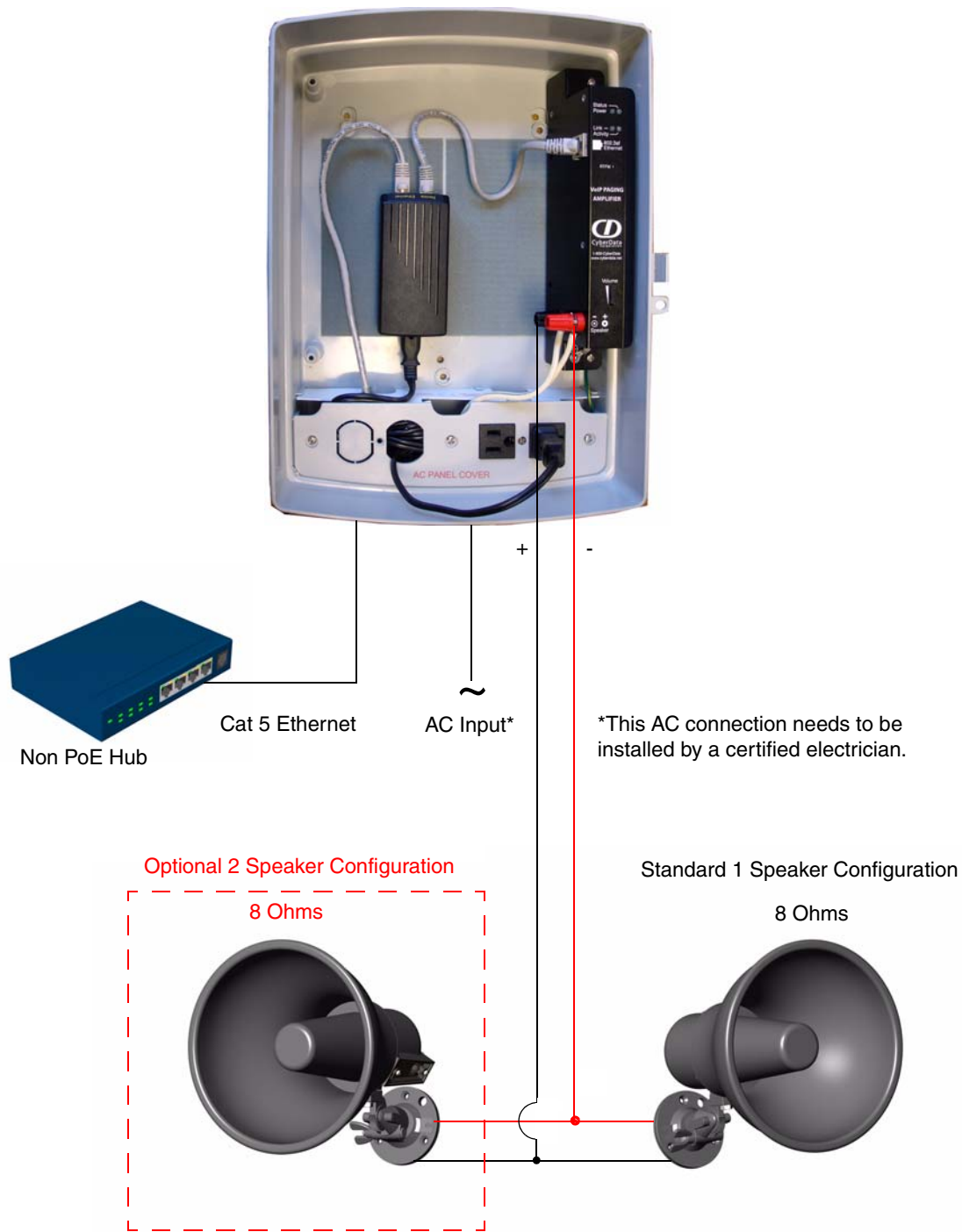
Figure 2-3. Connect a Loudspeaker
