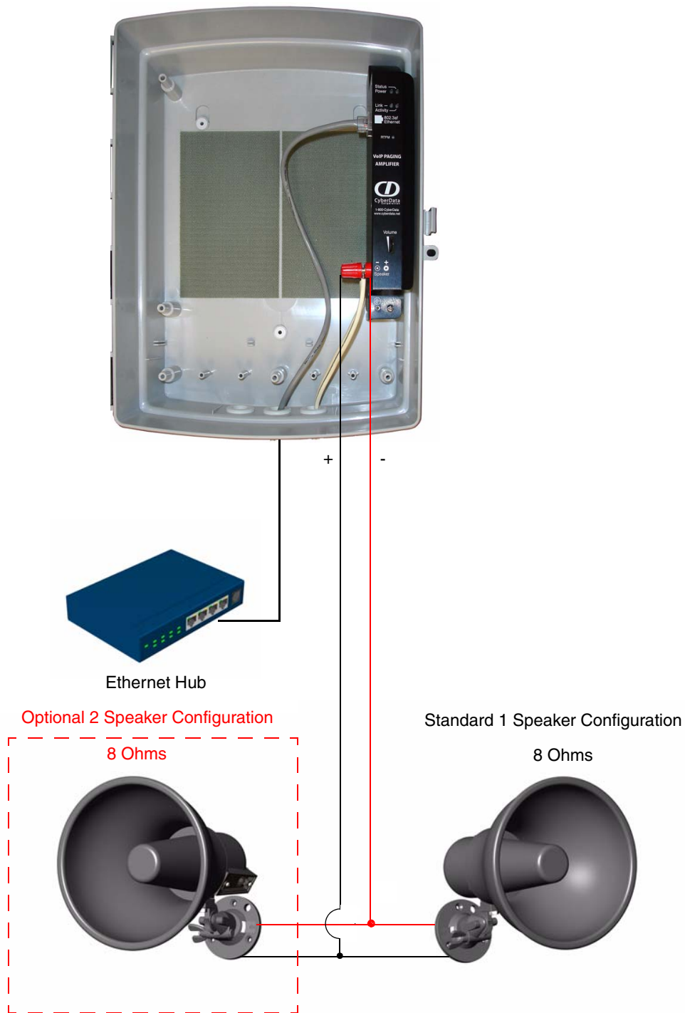
Figure 2-3. Connect a Loudspeaker
