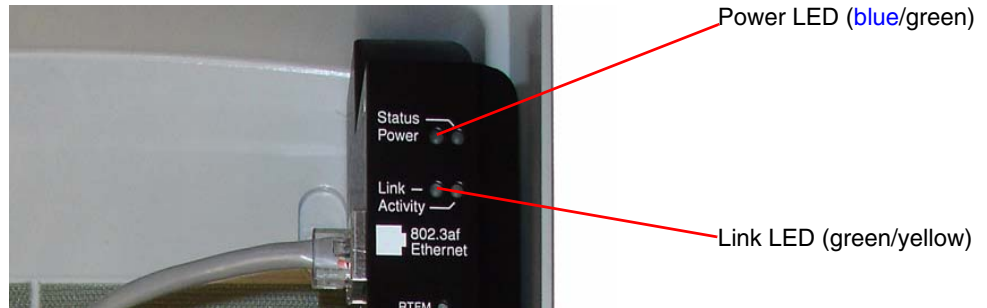
Figure 2-5. Loudspeaker Amplifier LEDs—Power and Link
