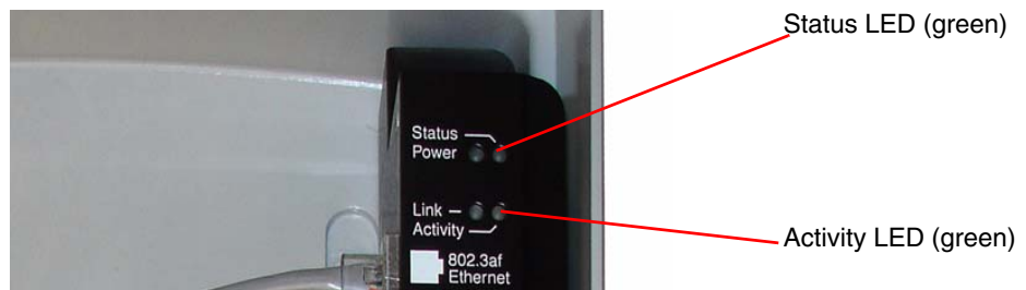
Figure 2-6. Loudspeaker Amplifier LEDs—Status and Activity
