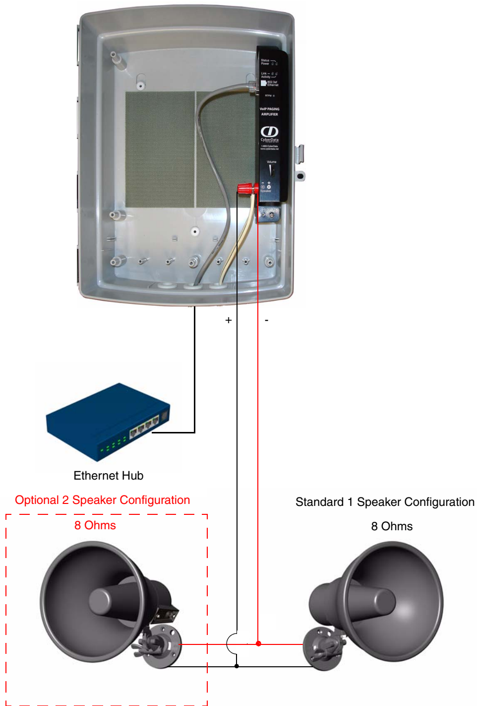
Figure 2-3. Connect a Loudspeaker
