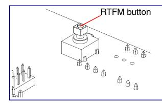
When the device is operational and linked to a network, you can use the Reset Test Function Management (RTFM) button to restore the device to the factory default settings.
