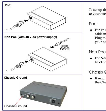
To set up the V2 Paging Server, connect the device to your network:
