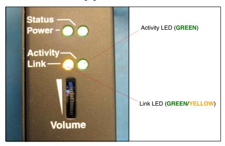
3.2. The GREEN power and status LEDs and the YELLOW link LED come on immediately. The activity LED illuminates GREEN for a 10Mb link or YELLOW/GREEN for a 100MB when the network link to the Paging Amplifier is established. The activity LED blinks to indicate network traffic.
