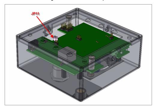
Figure 2-10. RTFM Switch Jumper
