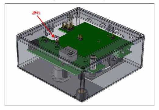
Figure 2-9. RTFM Switch Jumper
