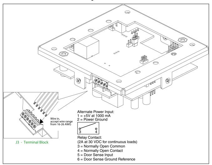
Figure 2-4. VoIP Intercom Connections
