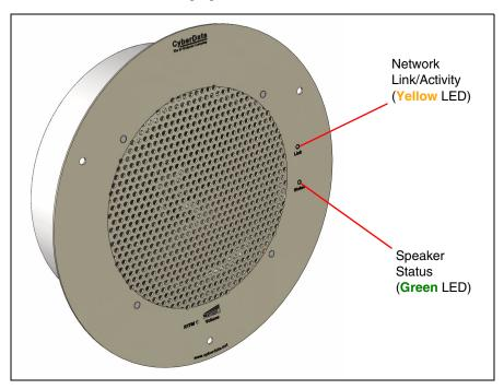
3.2. The **GREEN** power/status LED and the **YELLOW** network LED come on immediately. The **YELLOW** network LED will blink to indicate network traffic. After about 27 seconds, the **GREEN** power/status LED will blink twice to indicate that the board is fully booted.
