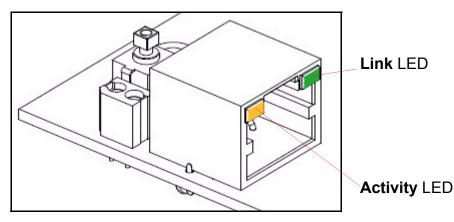
3.2. The GREEN Link LED blinks off once during the boot up process and then comes on again and remains constant (solid GREEN). The YELLOW Activity LED may be blinking depending on the network activity.
