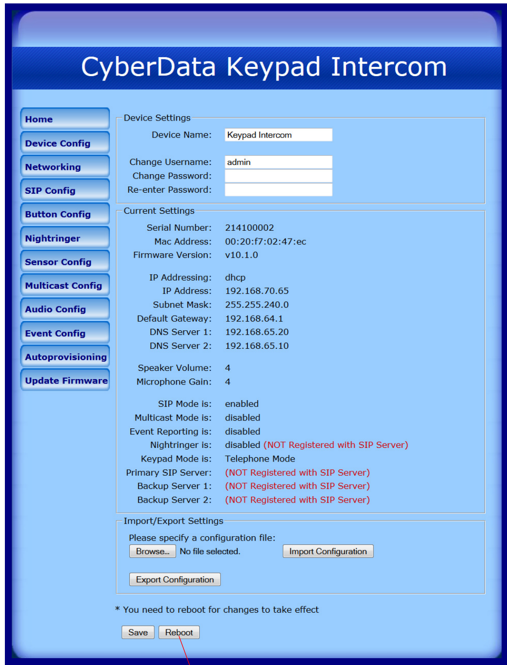
Figure 2-29. Reboot System Section
