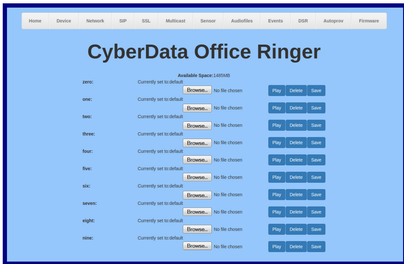
Figure 2-30. Audiofiles Configuration Page
