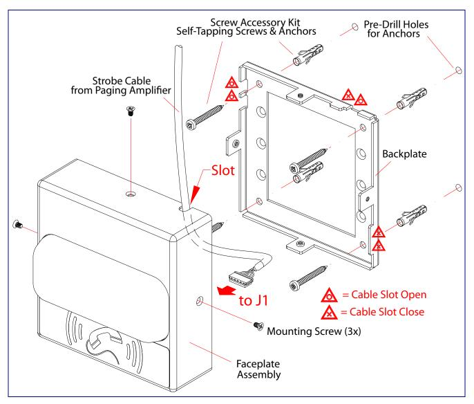
Figure A-2 shows the gang box mounting options for the Auxiliary RGB Strobe Kit.
