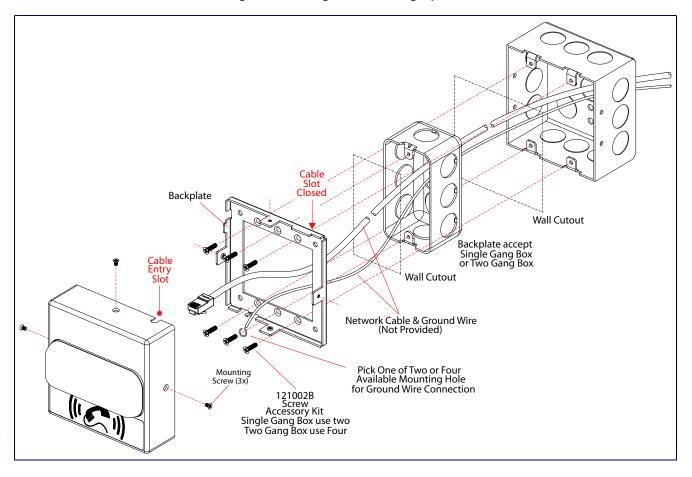
Figure A-3 shows the wall mounting with either a single or two gang box.
