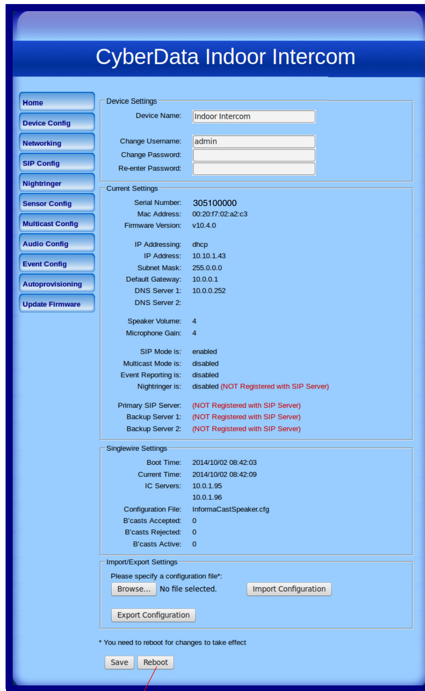
Figure 2-31. Reboot System Section
