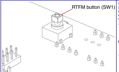
When the device is operational and linked to a network, you can use the Reset Test Function Management (RTFM) button (SW1 [see picture]) to announce the device's IP address or restore the device to the factory default settings.
