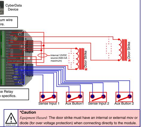
Equipment Hazard: The door strike must have an internal or external mov or diode (for over voltage protection) when connecting directly to the module.
