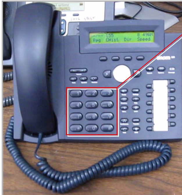
Figure 1-10. Talking and Listening Modes are Controlled by the Phone Keypad
