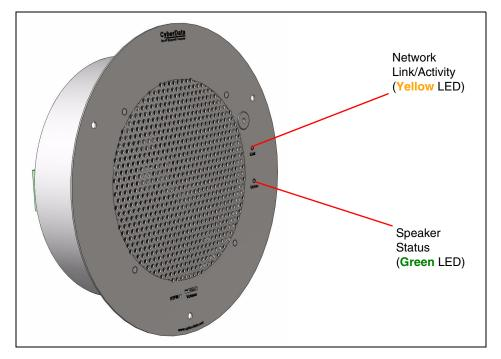
3.2. The GREEN power/status LED and the YELLOW network LED come on immediately. The YELLOW network LED will blink to indicate network traffic. After about 27 seconds, the GREEN power/status LED will blink twice to indicate that the board is fully booted.
