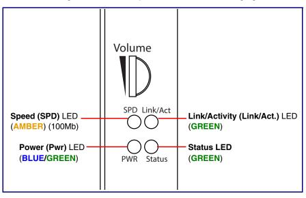
3.2. The **Power (Pwr)** LED is **GREEN** for 802.3af and is **BLUE** for 802.3at. The **GREEN Status** LED and the **GREEN Power (Pwr)** LED come on immediately. The **Speed (SPD)** LED illuminates **AMBER** for a 100Mb link or is off for 10MB when the network link to the device is established. The **Link/ Activity** LED blinks to indicate network traffic.
