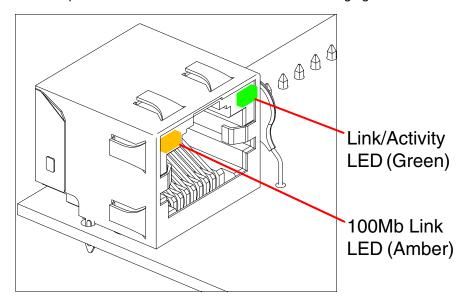
3.2. The green Link/Activity LED blinks off once during the boot up process when the device begins DHCP addressing and autoprovisioning attempts, and then comes on again and remains constant (solid green). The amber 100Mb Link LED may be blinking depending on the network activity.
