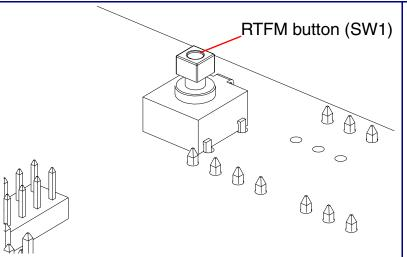
When the device is operational and linked to a network, you can use the Reset Test Function Management (RTFM) button (SW1 [see picture]) to restore the device to the factory default settings.
