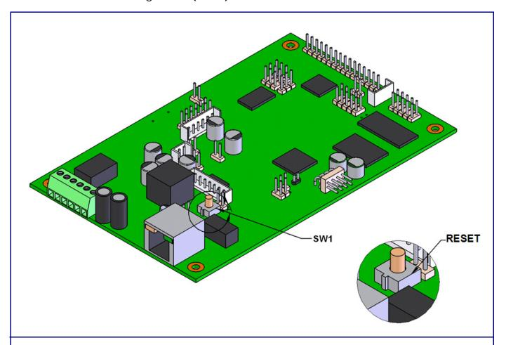
When the device is operational and linked to the network, use the Reset Test Function Management (**RESET**) switch on the board (see picture) to announce the device's IP address and test that the audio is working. During the IP address announcement, you will hear the IP address of your device through the handset receiver.
