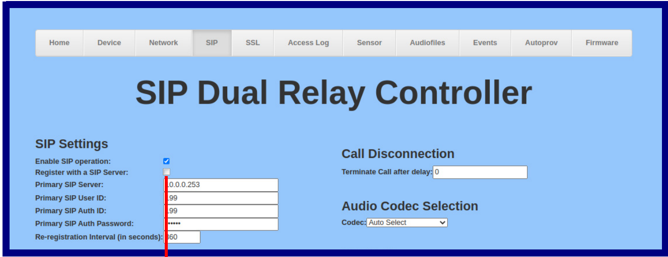
Figure 2-9. SIP Page Set to Point-to-Point Mode
