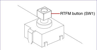
When the device is operational and linked to a network, you can use the Reset Test Function Management (RTFM) button to restore the device to the factory default settings.
