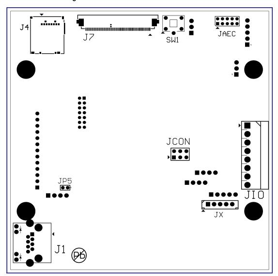
Figure 2-10. Connector Locations—Board Bottom
