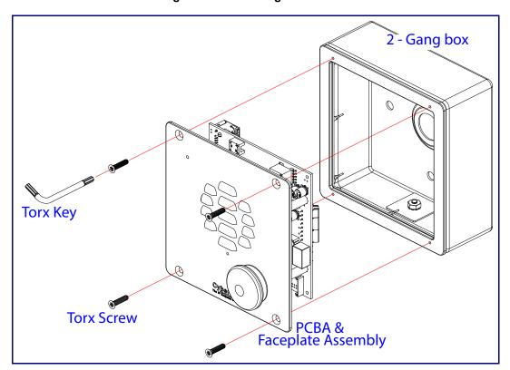
Figure A-10. Securing the Intercom
