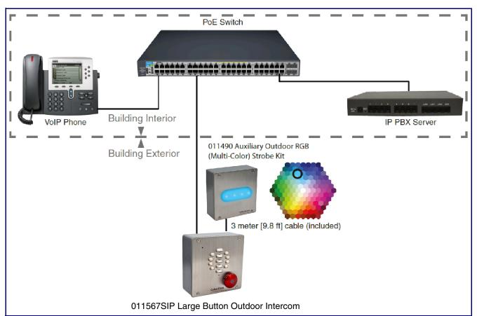
Figure 1-2. Typical Installation
