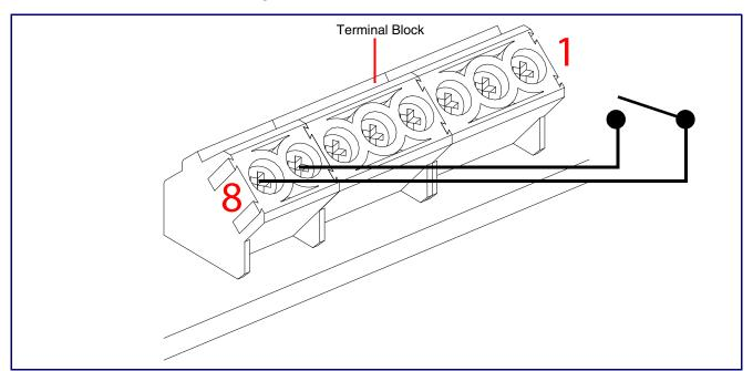
Figure 2-3. Remote Switch Connection
