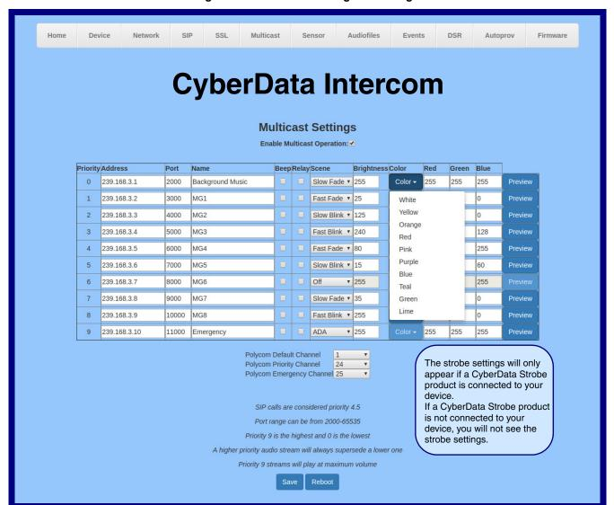
Figure 2-29. Multicast Configuration Page
