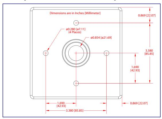
3.434 [87.23] 5.276 [134.00] 1.690 [42.93] ø0.280 [ø7.11] (4 PLACES) ø0.854 [ø21.69] - 3.380 [85.85] - 5.202 [132.13] 1.690 [42.93] Dimensions are in Inches [Millimeter] - 3.380 <sup>(85.85)</sup> 0.948 [24.07]
