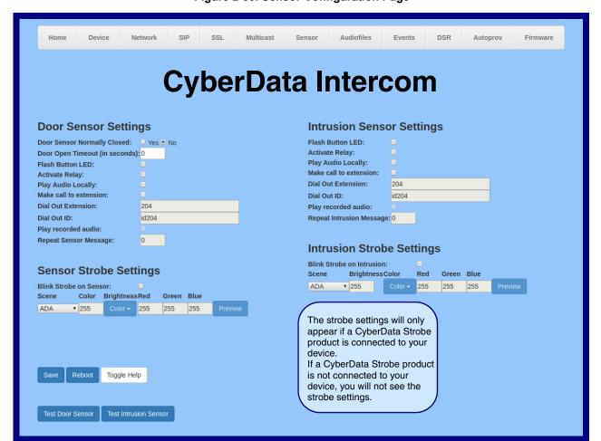
Figure 2-30. Sensor Configuration Page
