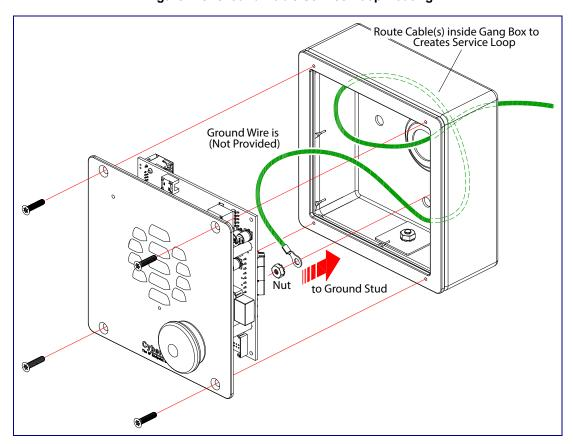
Figure A-8. Ground Cable Service Loop Routing
