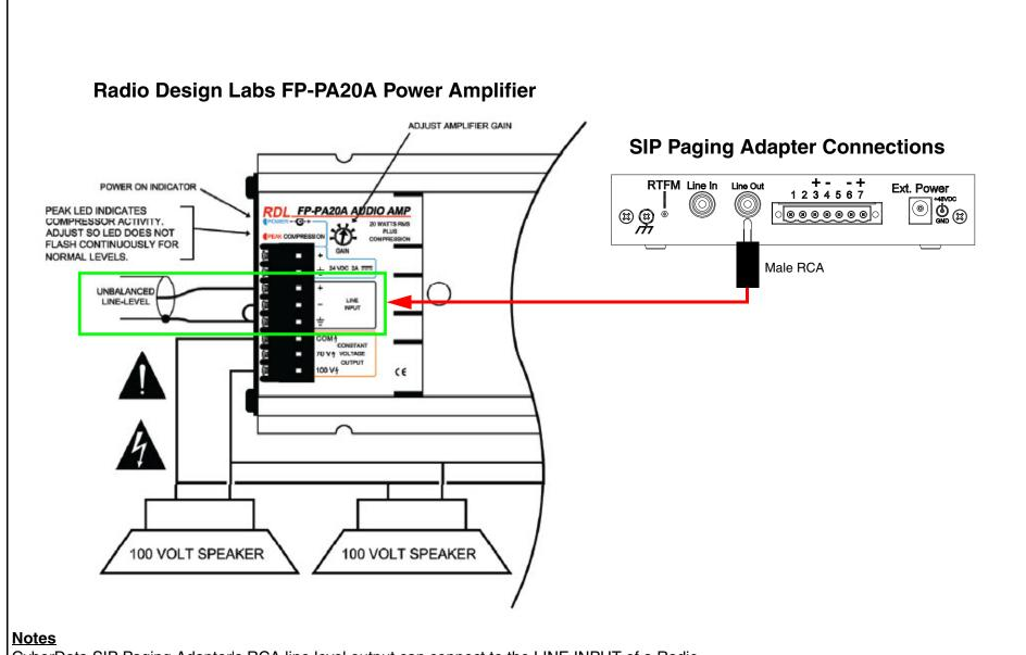
CyberData SIP Paging Adapter's RCA line level output can connect to the LINE INPUT of a Radio Design Labs (RDL) FP-PA20A Power Amplifier as an unbalanced connection. Use a 2-conductor, shielded RCA cable terminated on one end with a male RCA connector. The other end should be stripped for connection to the FP-PA20A Power Amplifier. Short the negative terminal pin to the ground terminal pin on the FP-PA20A Power Amplifier's terminal block per the diagram.
