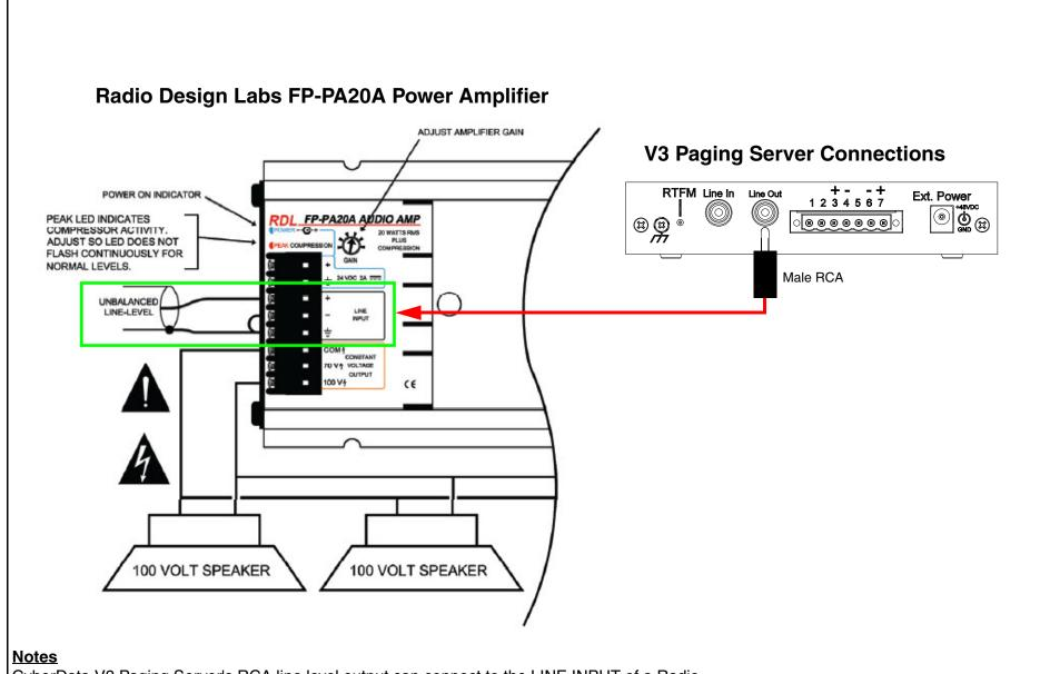
CyberData V3 Paging Server's RCA line level output can connect to the LINE INPUT of a Radio Design Labs (RDL) FP-PA20A Power Amplifier as an unbalanced connection. Use a 2-conductor, shielded RCA cable terminated on one end with a male RCA connector. The other end should be stripped for connection to the FP-PA20A Power Amplifier. Short the negative terminal pin to the ground terminal pin on the FP-PA20A Power Amplifier's terminal block per the diagram.
