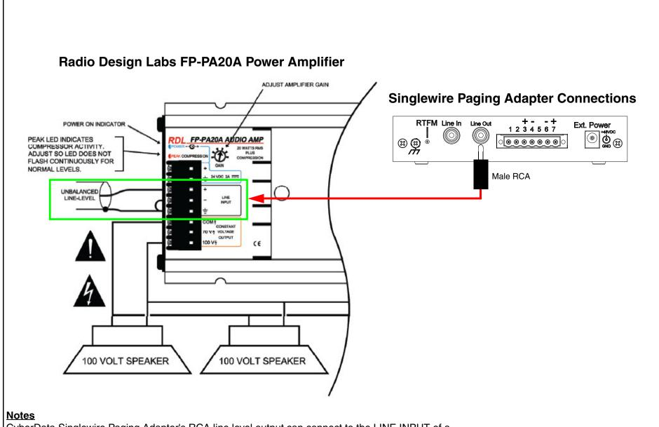
CyberData Singlewire Paging Adapter's RCA line level output can connect to the LINE INPUT of a Radio Design Labs (RDL) FP-PA20A Power Amplifier as an unbalanced connection. Use a 2-conductor, shielded RCA cable terminated on one end with a male RCA connector. The other end should be stripped for connection to the FP-PA20A Power Amplifier. Short the negative terminal pin to the ground terminal pin on the FP-PA20A Power Amplifier's terminal block per the diagram.
