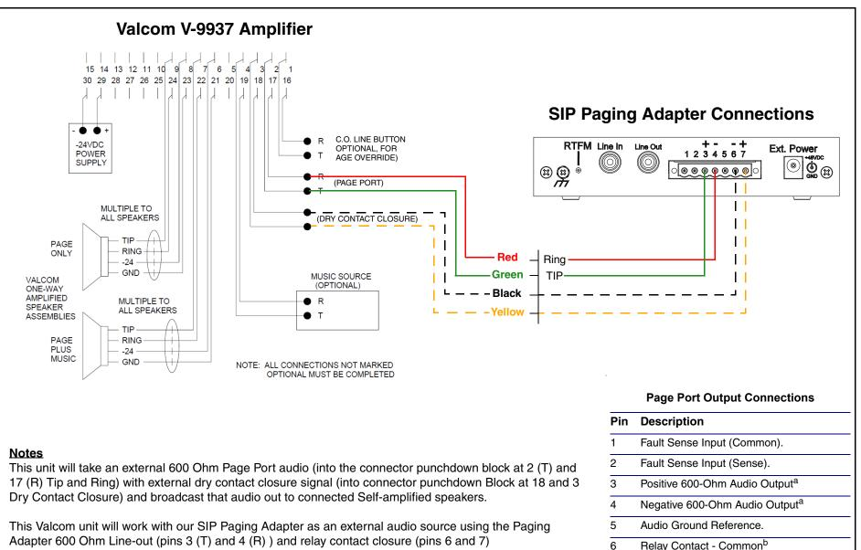
You will need to check "enable relay on local audio" on the SIP Paging Adapter Device Configuration page of the web interface. Please do not attempt to connect the Self-amplified speakers directly to our SIP Paging Adapter as this can damage the SIP Paging Adapter.
