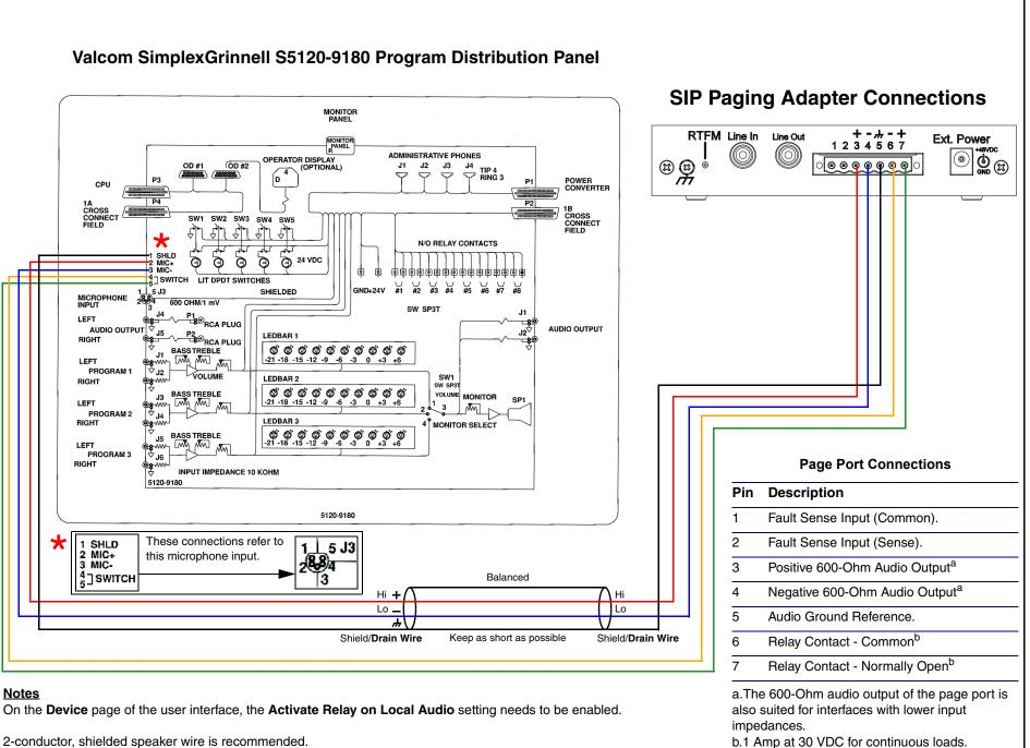
2-conductor, shielded speaker wire is recommended.
