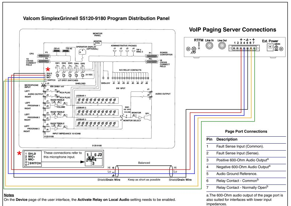
2-conductor, shielded speaker wire is recommended.
