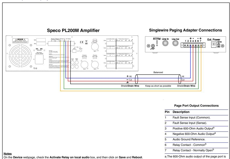
2 conductor, shielded speaker wire is recommended.
