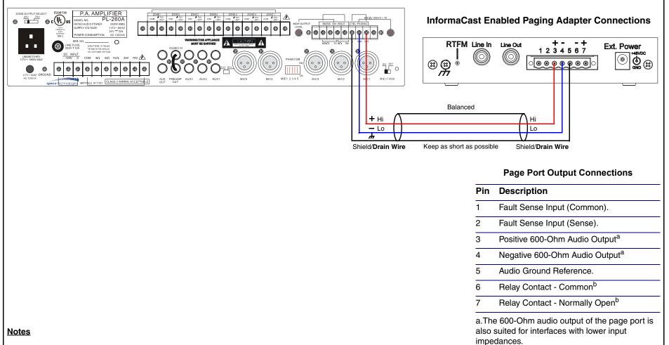
2 conductor, shielded speaker wire is recommended.
