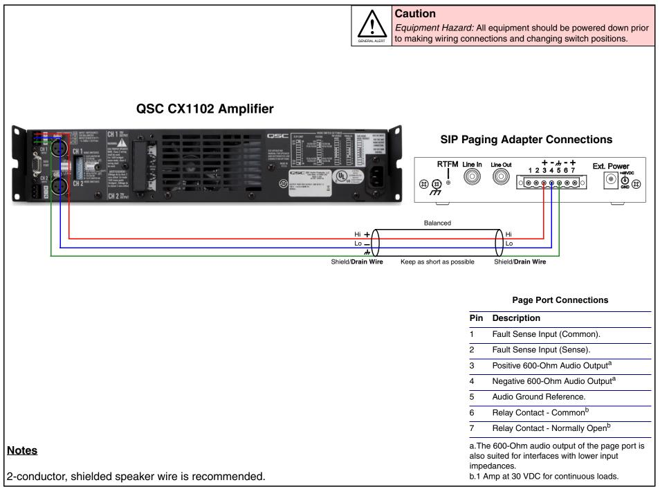
CyberData QSC CX1102 Amplifier to SIP Paging Adapter Connections
