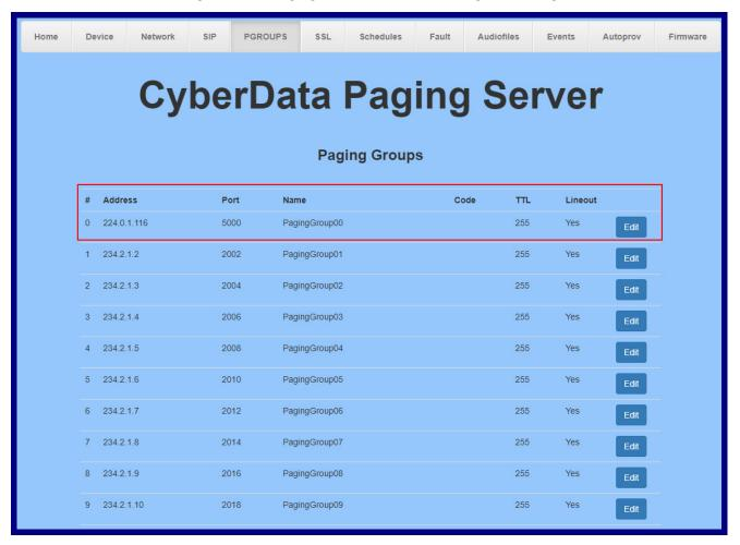
6. Enter the Polycom Multicast IP Address **224.0.1.116** (noted in step 5 of the Polycom Phone Configuration procedure) into the *Address* field under *Paging Groups*.
