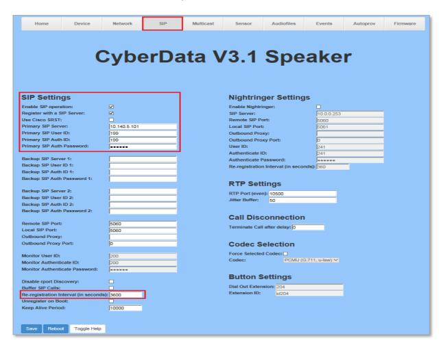
NOTE: The SIP Paging Server was powered up using the Ethernet port on the SIP Paging Server, via an Ethernet cable, connected to a PoE switch. DHCP is enabled by default on the CyberData SIP Paging Server. A DHCP server was used for the network parameters, and then manually provisioned the minimum configuration parameters required for validation with the ShoreTel Connect Onsite system.
