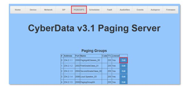
3. Define a **Name** for the Paging Group, and click on the **Save Changes** button. Make note of the **Address** and **Port** number, as they will be used in the SIP Speaker configuration.
