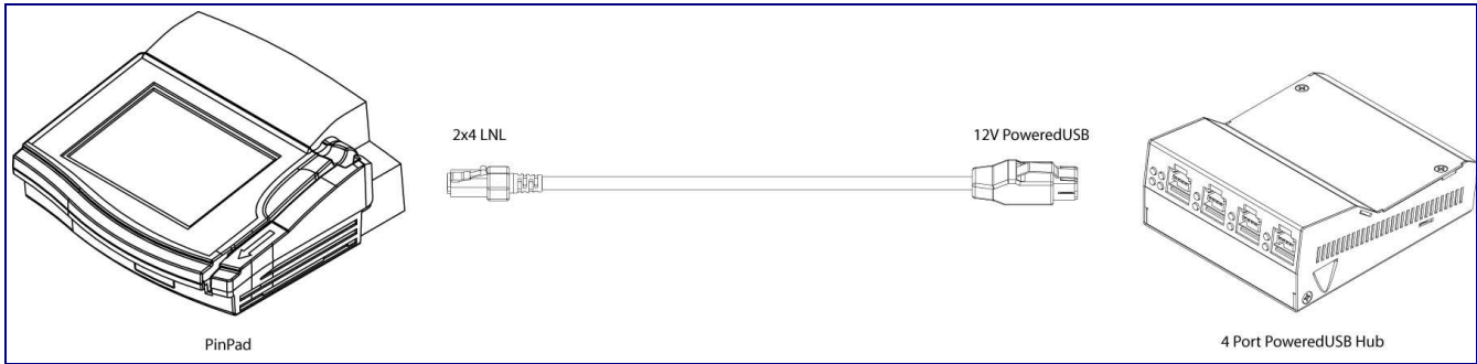
Figure 2-11. Cable, +12V PoweredUSB to 2x4 PoweredUSB
