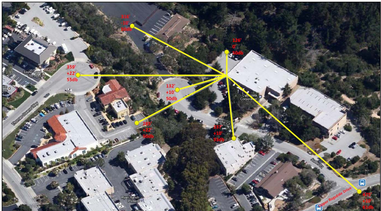
Figure 2. Distance and Elevation from the Speakers that Intelligible Notifications can be Heard
