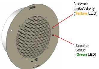
3.2. The **GREEN** power/status LED and the **YELLOW** network LED come on immediately. The **YELLOW** network LED will blink to indicate network traffic. After about 27 seconds, the **GREEN** power/status LED will blink twice and the speaker will beep to indicate that the board is fully booted. You can disable **Beep on Initialization** on the **Device Configuration** page.
