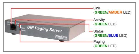
3.2. The **GREEN/BLUE Status** LED and the **GREEN Paging** LED both blink at a rate of 10 times per second during the initial network setup.
