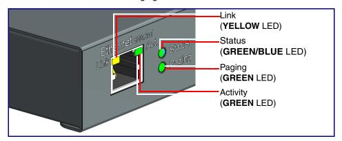
3.2. The **GREEN/BLUE Status** LED and the **GREEN Paging** LED both blink at a rate of 10 times per second during the initial network setup.
