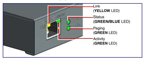
3.2. The **GREEN/BLUE Status** LED and the **GREEN Paging** LED both blink at a rate of 10 times per second during the initial network setup.
