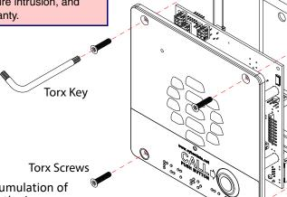
Properly seal the intercom to prevent the accumulation of dust and moisture. Critical areas are shown in the image above: the conduit hole, all screw holes and an application of sealant around the perimeter.
