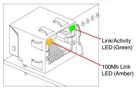
3.2. The green **Link/Activity** LED blinks off once during the boot up process when the device begins DHCP addressing and autoprovisioning attempts, and then comes on again and remains constant (solid green). The amber **100Mb Link** LED may be blinking depending on the network activity.
