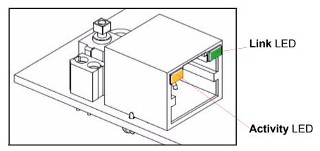
3.2. The GREEN Link LED blinks off once during the boot up process and then comes on again and remains constant (solid GREEN). The YELLOW Activity LED may be blinking depending on the network activity.
