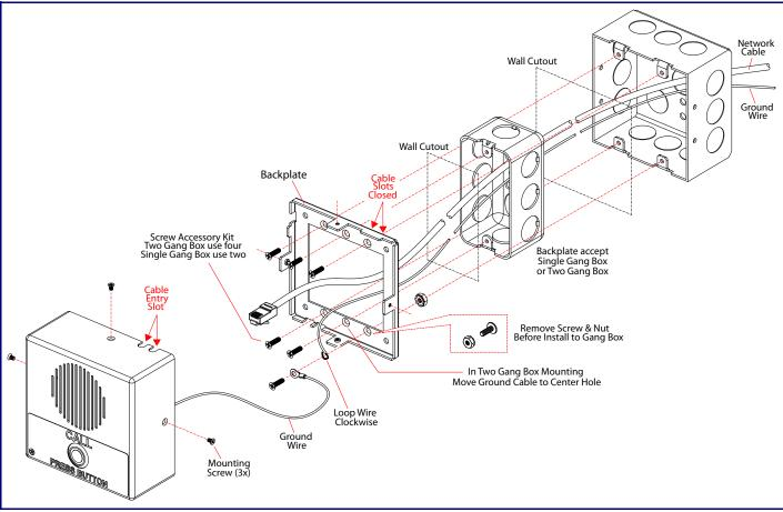
CyberData Installation Quick Reference The IP Endpoint Company SIP Indoor Intercom SIP Compliant 011211\*, RAL 9003, Signal White \*Replaces the 011111 number.
